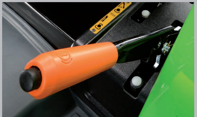
Mechanical automotive-style parking brake near the operator for easy reach.
