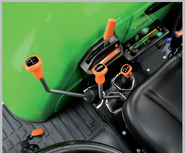
Transmission controls, foot and handle throttles, rear 3-point hitch and hydraulic controls are all within easy reach to the right side of the seat. (4080E).
