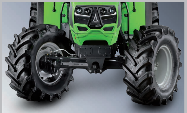
The compact chassis and smart axle design allow for a steering angle of up to 55 degrees.
