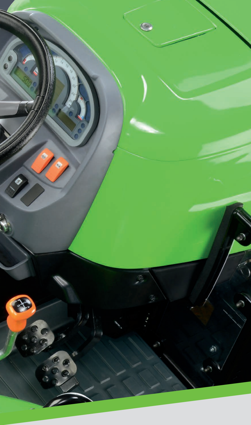
The new information display in the front dash keeps the operator informed about the machine's status and operation.
