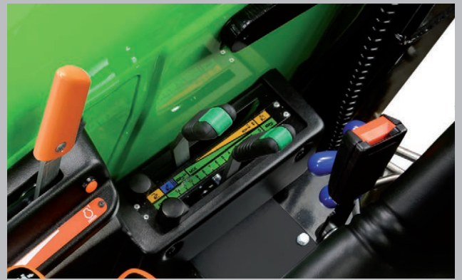
The rear 3-point hitch is mechanically operated with simple, familiar controls.
