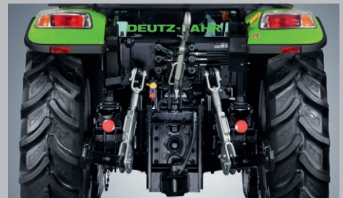
13.2 gpm hydraulic pump, up to three control valves, 5500 lbs rear power lift, 540 PTO.
