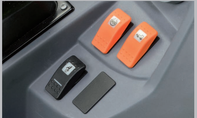
Electro-hydraulic activation of the 4wd and differential lock.
