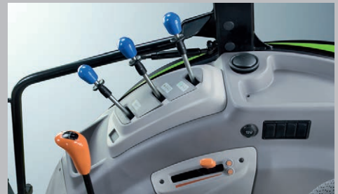
Mechanical transmission with up to 15 x 15 gears, 25mph at 1,870 rpm.
