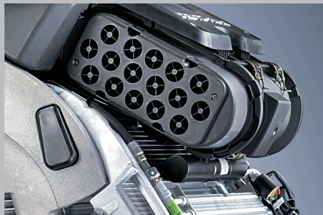
Pre-cleaning system of the air intake filter: spiral tubes and an aspirator hose removes 95% of the dust before entering the primary filter.
