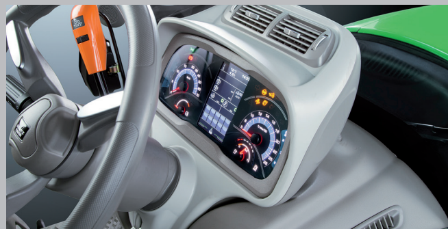
State-of-the-art dashboard cluster with new InfoCentre Pro : 5" high-res LCD color display for customizable top information concept.
