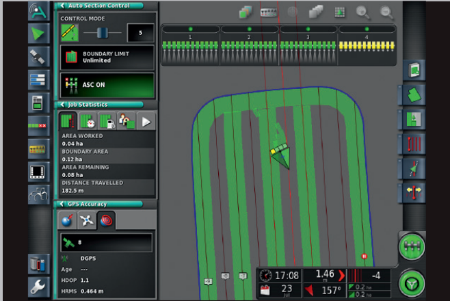
Section control/ variable rate control as standard.
