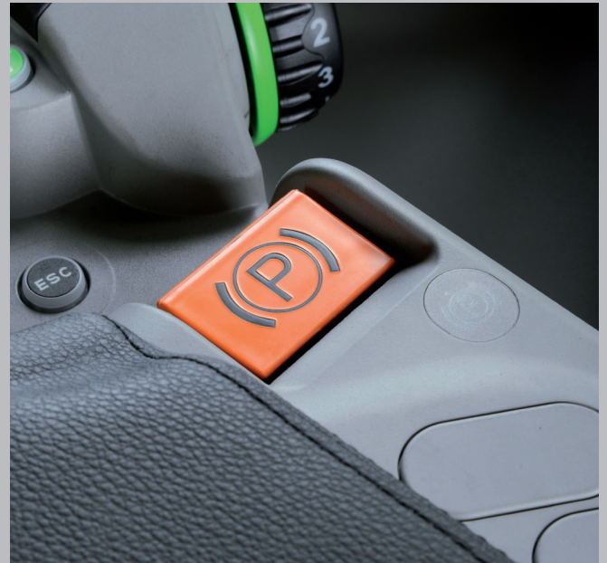
TTV models - EPB replaces the handbrake lever and is operated via an electric push-button control on the armrest console.
