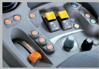
PTO controls (front/rear) are conveniently integrated in the armrest...
