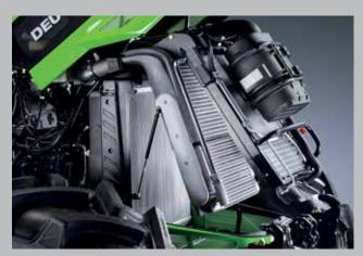
Newly designed cooling system. Fully openable for easy maintenance.
