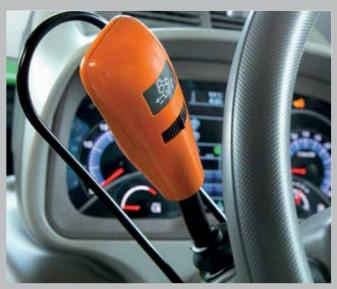
PowerShuttle with SenseClutch - 5 levels of reversing sensitivity that can be easily adjusted.
