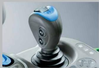
Auxiliary valves are controlled via a joystick with an integrated smart wheel.
