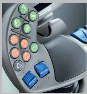
Up to 4 cruise speeds can be memorised to optimise application and efficiency.
