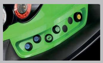
External control for auxiliary hydraulics, rear lift and PTO mounted on both sides of the tractor.
