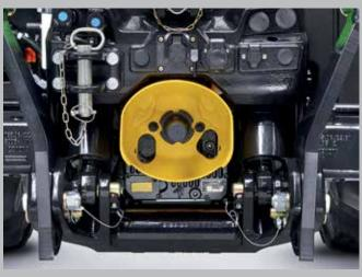
Up to 5 proportional spool valves at the rear and 2 in the front. Front lift integrated to the tractor and closer coupled
