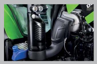
SCR aftertreatment system and passive DPF (diesel particulate filter) for saving fuel and operating costs.
