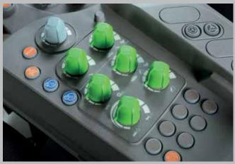
... along with the front and rear lift controls.
