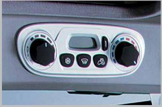
Pre-select temperature; the automatic controls precisely regulate the air flow.
