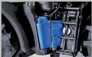
159 gal diesel and 14 gal DEF are sufficient for more than one day of hard work in the field.
