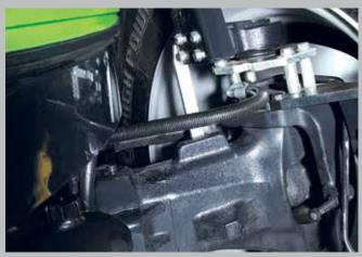
Front axel. Maximum spring effect and a steering angle of up to 50 degrees.
