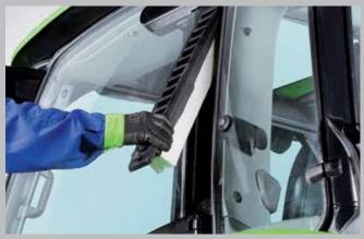
The cab air filter in the cab post can be easily accessed without tools.
