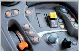
The PTO settings and activation are conveniently integrated into the armrest ...
