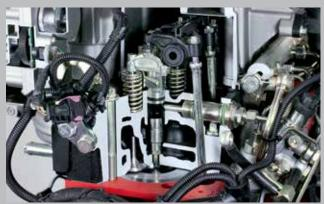
DCR technology. 29,000 PSI injection pressure ensures maximum engine efficiency.
