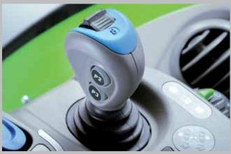
Three hydraulic valves can be controlled via a simple joystick with integrated smart wheel.
