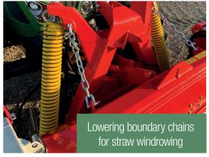
For use in **straw**, the working unit can be locked via lowering chains and so be carried over ground. No constant contact with the ground, less dust formation, stones remain on the ground, less wear on the sliding discs (low heating, no flying sparks) and on the tines.
