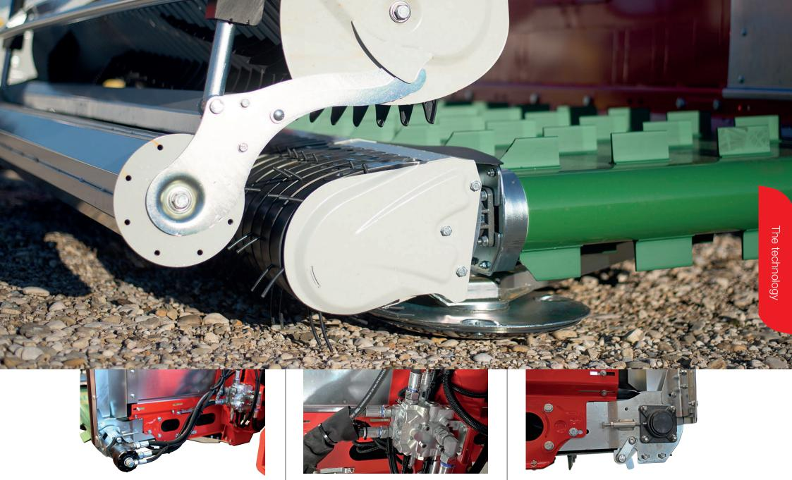
Belt drive is via hydraulic motor OMR with leakage oil line - a coupling for tension-free drive sits in between.
