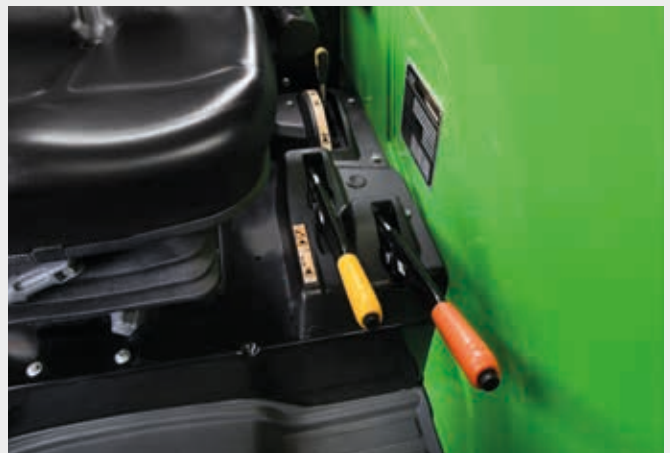
↑ Mechanical PTO speed selector and engagement.
